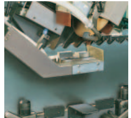
The saw blade support with automatic height adjustment guarantees a precisely horizontal position of the saw blade (Fig. CA 300)
