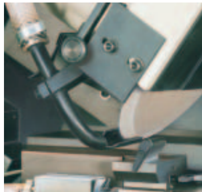
Automatic dressing of the corundum grinding wheel as an optional feature (Fig. CA 200)
