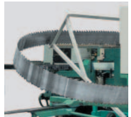
Bracket to simplify the insertion of saw blades (Fig. CA 300)
